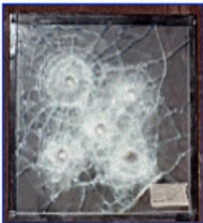
Post Test Impact Side Dual Pane Glazing 2 Inside
