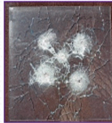
Post Test Impact Side Dual Pane Glazing 1 Outside
