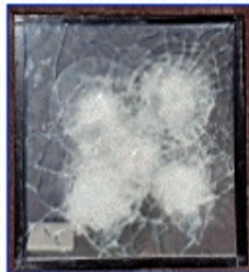
Post Test Rear Side Dual Pane Glazing 2 Inside
